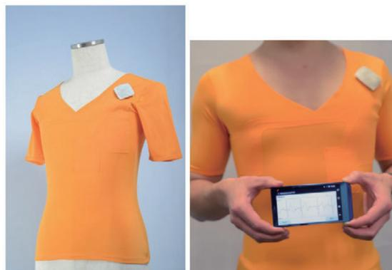
Shirt with "hitoe" and example of ECG (electro cardio gram) monitoring.
