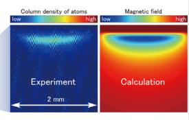
NTT BRL succeeded in trapping rubidium atoms in a magnetic potential generated from a persistent supercurrent on an atom chip. This is the first step for the single atomic device.
