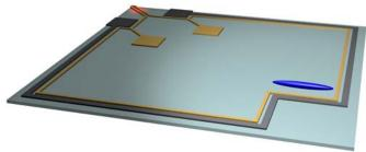
Persistent supercurrent atom chip, that NTT BRL achieved for the first time, is practically noise free and expected to trap single atoms with maximum flexibility.
