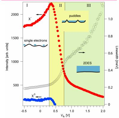
Electrons are induced as  $V_{fb}$  increases. The "electron puddle state" (regime II) is observed in between the single electron localized state (I) and the two-dimensional electron system (III)
