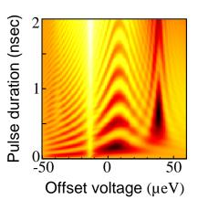
Multi-functional quantum information processing device fabricated by using GaAs/AlGaAs heterostructure (upper left), Simulation of correlated coherent oscillations (upper right)
