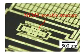
MEMS power generator fabricated by low-temperature thick-film process
