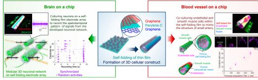
(Upper left) Staining image of encapsulated 3D neuronal aggregate and representative recorded neuronal signal (Lower left) Schematic images of self-folding electrode array and modular 3D
