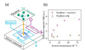
(a) Overview of magnetometry system using a superconducting flux qubit for measuring electron spins in biomaterials.
