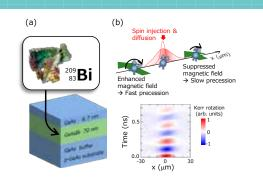
(a) Schematic structure of sample in which Bi atoms are incorporated in GaAs (b) Spatiotemporal mapping of the magneto-optical Kerr effect. The spin precession frequency, which appears as red and blue oscillations, changes with the probe position x, as a result of the enhanced spin-orbit interaction.
