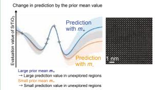
(Left) Change in prediction due to the prior mean value (Right) Electron microscopy image of a stoichiometric SrTiO<sub>3</sub> thin film
