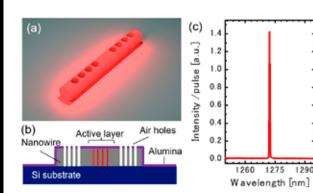
(a)Nanostructure-implemented nanowire laser (b) Cross-sectional view of the nanowire (c) Lasing spectrum
