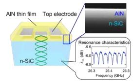
Schematic of the acoustic-impedance matched GHz acoustic device (left). Crosssectional SEM image (upper right) and resonance characteristics (lower right) of the device.
