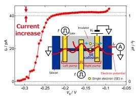
Pump current during single-electron collisions. The current exceeded the current generated from the left pump (elementary charge  $e \times \text{clock}$  frequency f). Inset: Schematic diagram of the device and part of the electrical measurement system.
