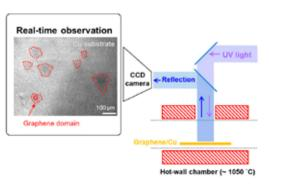
Schematic illustration of real-time optical observation system for thermal CVD (right) and optical reflection micrograph of graphene on Cu substrate (left).
