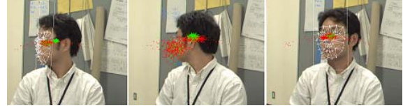
Figure 10. Successful recovery from tracking failure (12 frame interval between above images).
