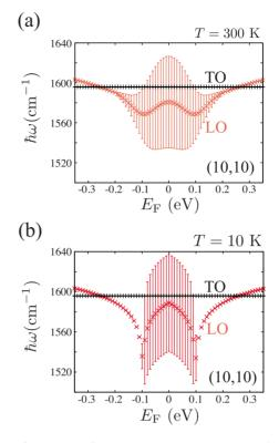
FIG. 2. (Color online) The  $E_F$  dependence of the LO (red curve) and TO (black curve) phonon energy in the case of the (10,10) armchair nanotube. (a) is taken at room temperature and (b) is at 10 K. Only the energy of the LO mode is shifted, with the TO mode frequency being independent of  $E_F$ . The decay width ( $\Gamma_{\lambda}$ ) is plotted as an error bar.
