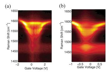
FIG. 8. (Color online) Experimental results for the Raman G-band intensity as a function of applied gate voltage for two metallic SWNTs (a) and (b). A strong (weak) intensity peak is denoted by the yellow (black) color.
