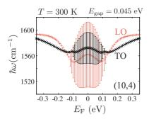
FIG. 6. (Color online) The  $E_F$  dependence of the LO (red curve) and TO (black curve) phonon energy for the (10,4) metallic chiral nanotube.  $E_{gap}$  denotes the curvature-induced minienergy gap which has the same value as that for the (15,0) tube in Fig. 4(a). The difference between the behavior of the (10,4) and (15,0) nanotubes comes from the fact that the phonon eigenvector of the LO (TO) mode is not pointing along the tube axis in the case of the (10,4) tube.
