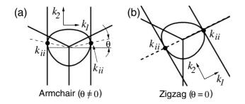
FIG. 7. Trigonal warping effect of an equienergy surface in the 2D Brillouin zone and cutting lines for (a) armchair and (b) zigzag nanotubes. In the case of (a) armchair nanotubes, the  $\theta$  value defined from the  $k_1$  axis in Fig. 5 is not zero while in the case of (b) zigzag nanotubes,  $\theta$  is always zero, which explains the chirality dependence of the relative Raman intensity of LO and TO phonon modes.
