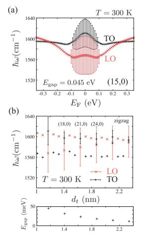
FIG. 4. (Color online) (a) The  $E_F$  dependence of the LO (red curve) and TO (black curve) phonon frequency for a (15,0) zigzag nanotube. Not only the frequency of the LO mode but also that of the TO mode is shifted due to the curvature effect. (b) The diameter  $d_t$  dependence of the phonon frequency for zigzag nanotubes, including zigzag semiconducting tubes.  $E_{gap}$  denotes the curvature-induced minienergy gap.
