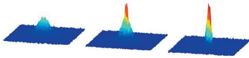
Time of flight images are taken after 16ms along gravitational axis.
